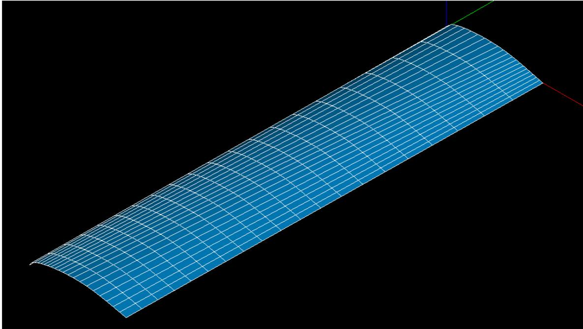
You can see that the mesh is not good, it is given by the fact that the **inner** edge has another orientation than the tip edge. It is easy to correct it.
