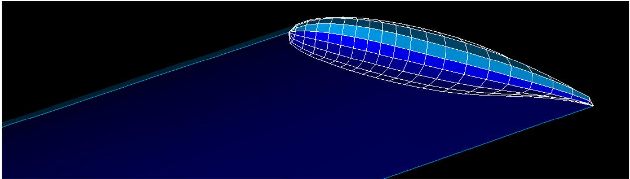
You can see that the **tip\_down** mesh has another color. The **dark blue** means that you are seeing the inner part of the patches. We need to change the orientation of this mesh in order to have it correct:
