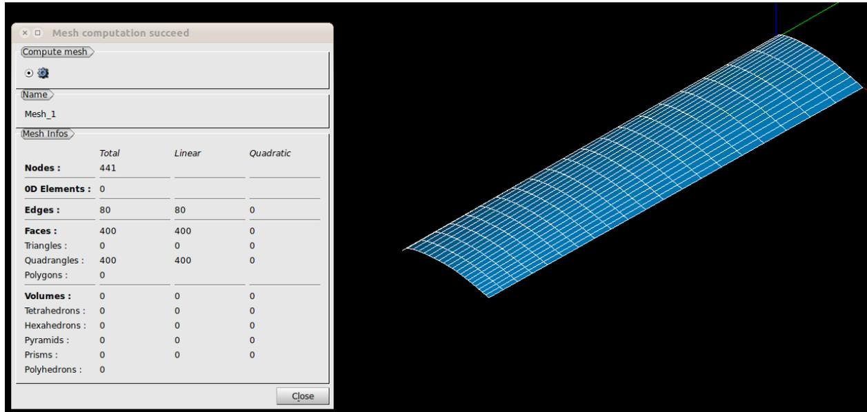
The four edges of the mesh boundary are meshed with the same hypothesis, **span\_normal**, which is intended to satisfy our requirements along the span. It is now it is necessary to define precisely the parameters for the boundaries representing the wing profile.
