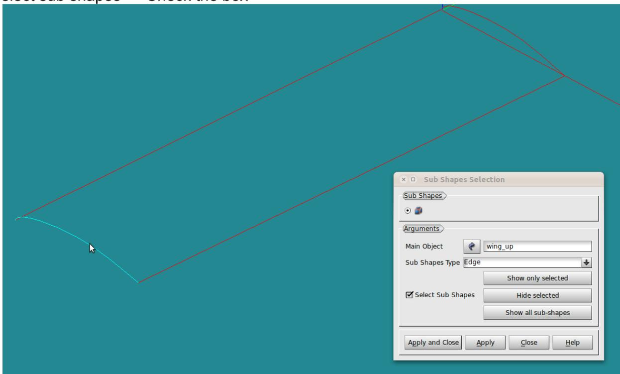
Select the edge of the wing section close to the wing tip, then apply.
