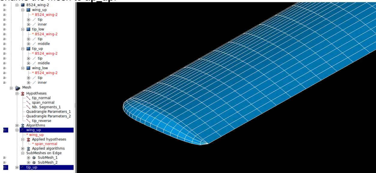
The two meshes are fitting together. In order to easily see the discretization on the graphic display, select the meshes on the object browser (maintain CTRL pressed in order to select several meshes).
